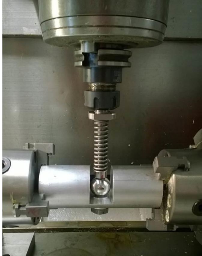
Figure B3: Titanium alloy scrape setup in CNC mill.
